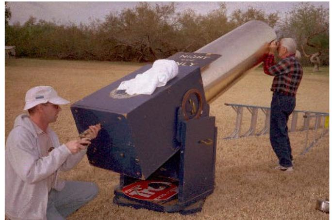
*John Dobson (right) checks the collimation.
