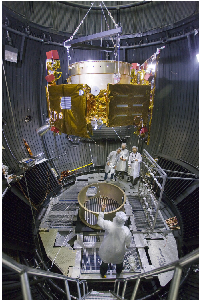
Technicians at Northrop Grumman gently maneuver the LCROSS spacecraft into the thermal vacuum chamber. Credit: NASA, courtesy of Northrop Grumman.
