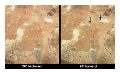
Two cameras on MISR made these images of the same part of the Mojave Desert. The camera pointed at an angle of 26 forward saw the flashes from two solar electric power generating stations. These objects are nearly invisible at the other angle.
