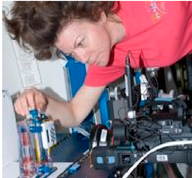
Astronaut Cady Coleman performs a Capillary Flow Experiment interior corner flow test.
